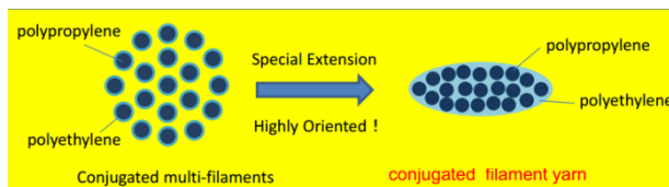
Scheme 1: Transformation of conjugated filaments into yarn by heat
