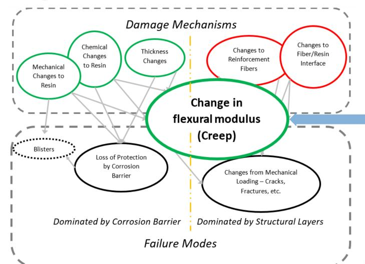
ULTRAAnalytix measures changes in laminate flexural modulus
