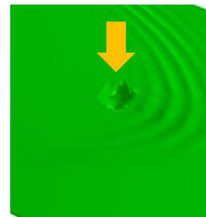
Fatigue crack detection with lamb waves
