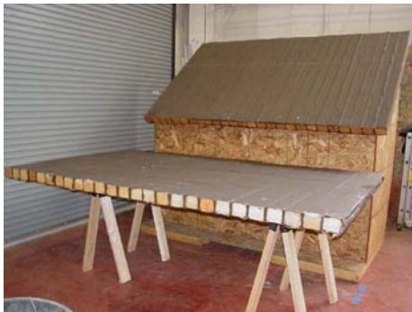
FIGURE 14: Biobased composite roof panels; one of them is mounted on a demonstration house made of timber [184].
