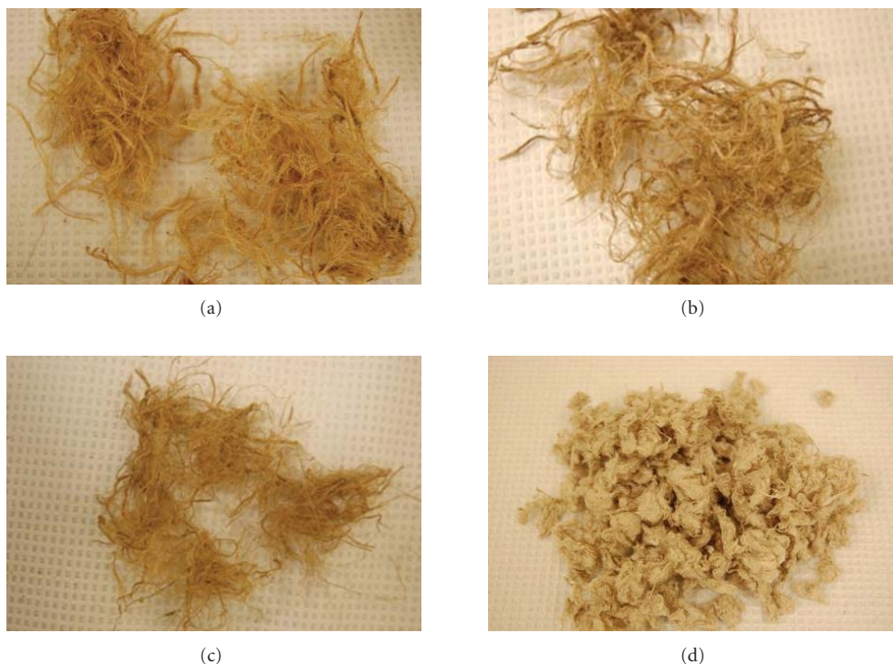
FIGURE 1: Images of the fibers digested at (a) 80°C, (b) 110°C, (c) 130°C, and (d) 160°C.
