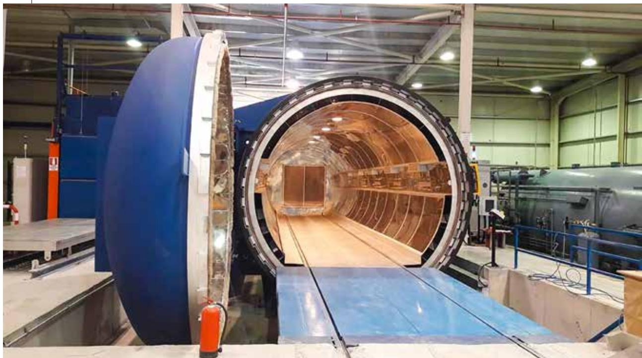
Composite Autoclave - Ø3600 x 14000 mm usable dimensions Approved & Actively working for Aerospace Industry
