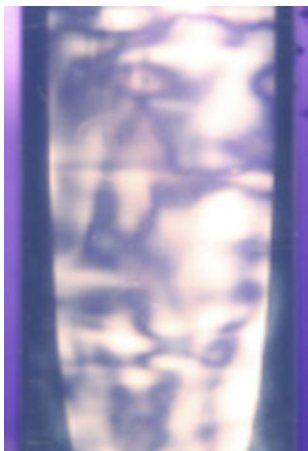
Fig. 12 CNC suspension shows birefringence between crossed polarizers (Petersson et al. 2007)
