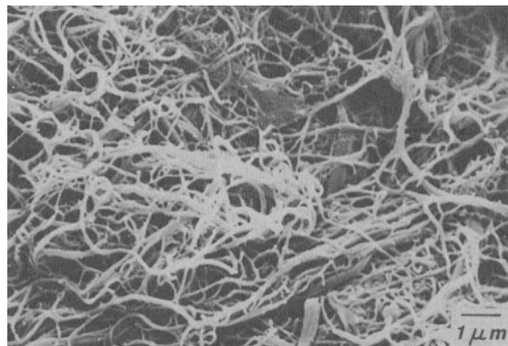
Fig. 6 SEM micrograph of microfibrillated cellulose (MFC) (Turbak et al. 1983)
