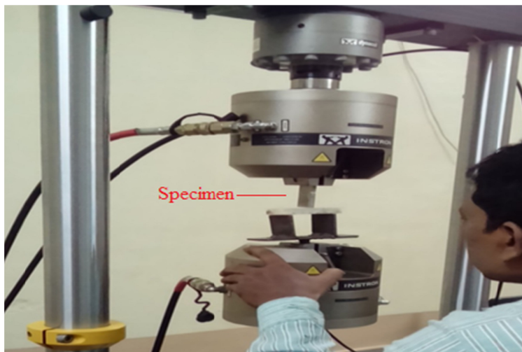
Figure 2 Flexural test on Glass Composite
