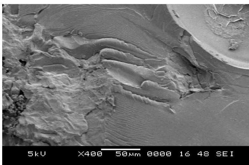
Figure 14. Crushed matrix surface of the epoxy composite.
