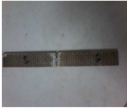
Figure 7: Flexural Tested Specimens.
