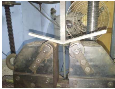
Figure 8: Flexural Tested Specimen at Failure.
