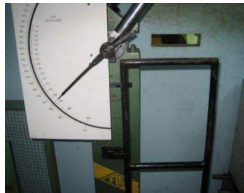
Figure 11: Charpy Test/Impact Test Set Up.
