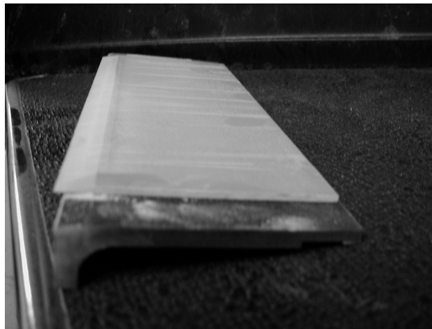
Taper produced on Tabbing strip
