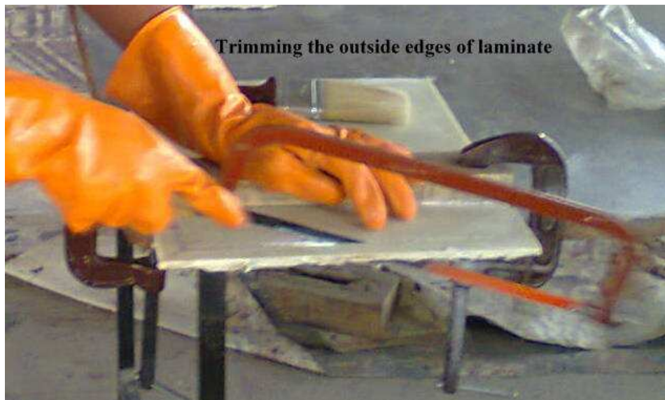
Trimming the edges of Cured Laminate
