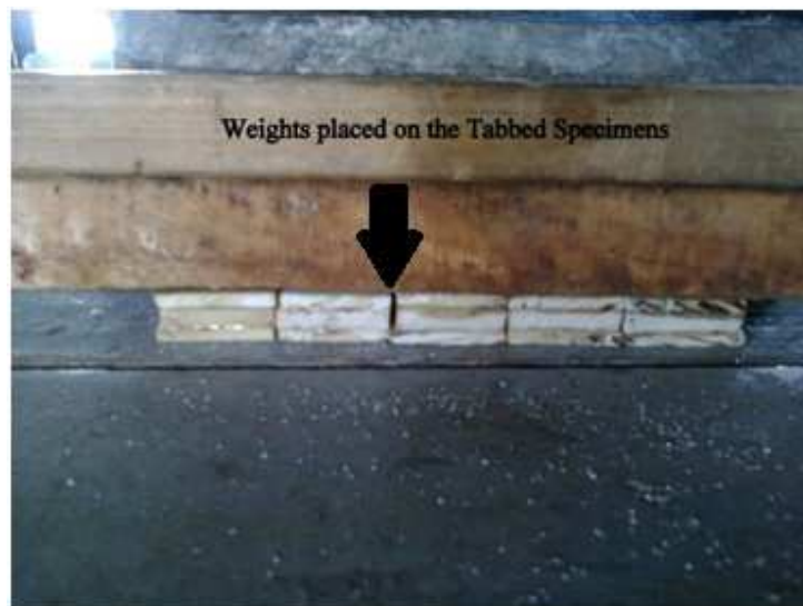
Weights placed on tabbed specimens
