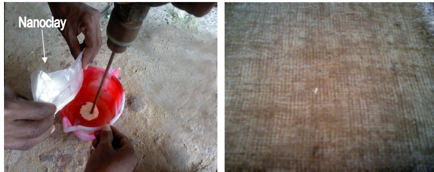
Fig. 1. Preparation of nanocomposites by hand lay-up process.
