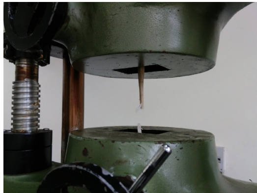
Figure 8: Broken Sample after Tensile Test
