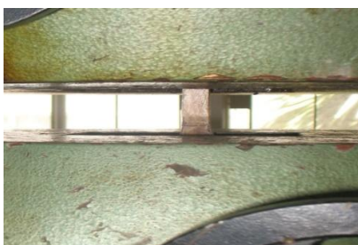
Fig -2: Tensile specimen in UTM
