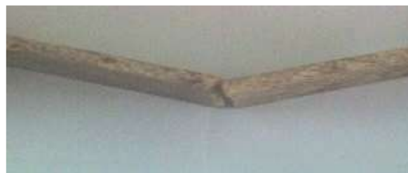
Fig 13: Flexure tested specimen
