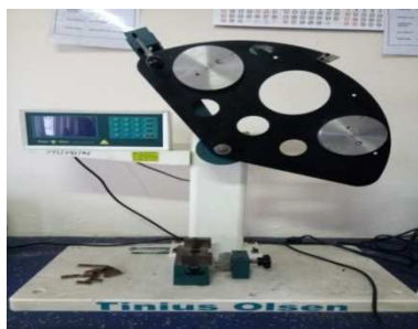
Figure 6: Izod Impact Test
