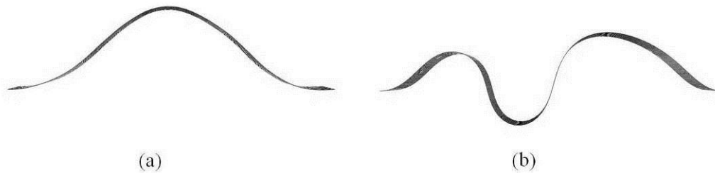
Fig. 21 FE model of a fabric sample compressed from each side with (a) high bending stiffness and (b) low bending stiffness
