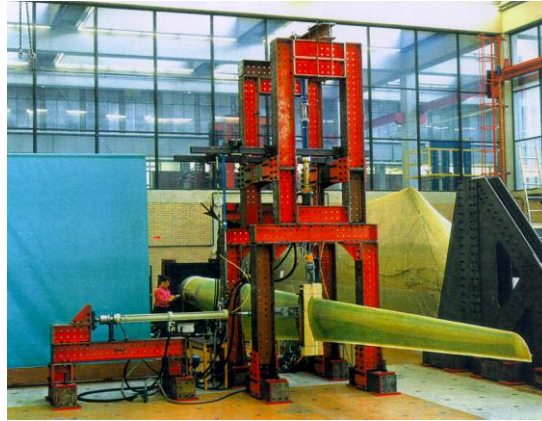
Fig. 15 Dual-axis test set-up using hydraulic actuators
