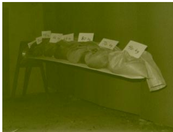
Fig. 4 The early experience of static blade testing using sandbags
