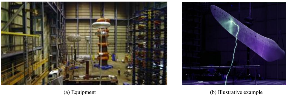
Fig. 20 Overview of equipment for blade lightning strike testing and an illustrative example
