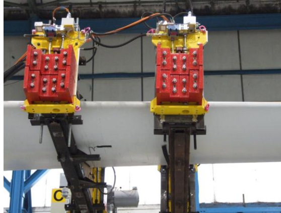
Fig. 14 Narec's compact resonant mass (CRM) system
