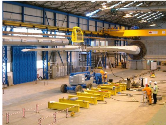
Fig. 12 Narec's first fatigue testing equipment – a resonant mass system powered by hydraulics
