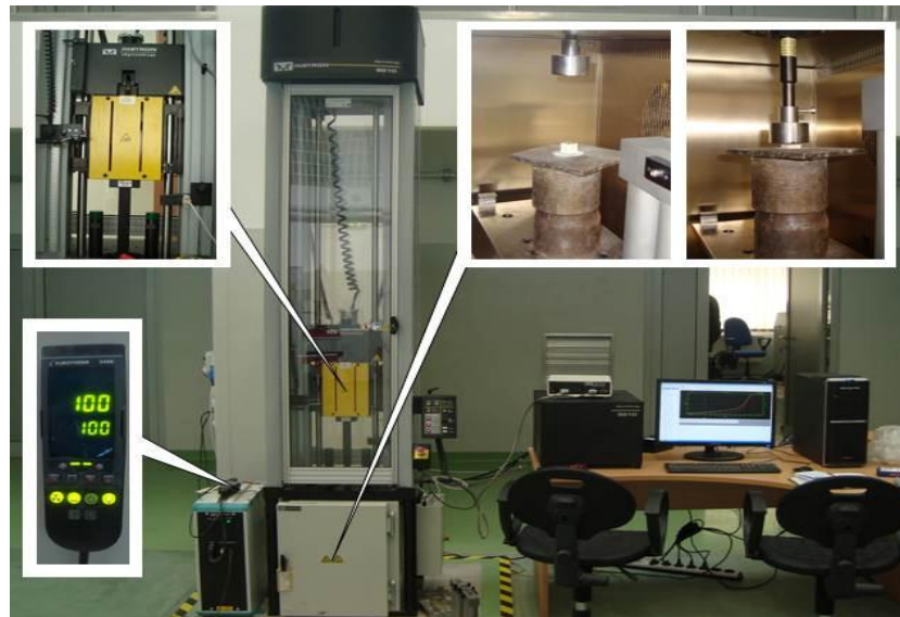
Fig. 14 A Instron – Dynatup 40 kN impact testing machine
