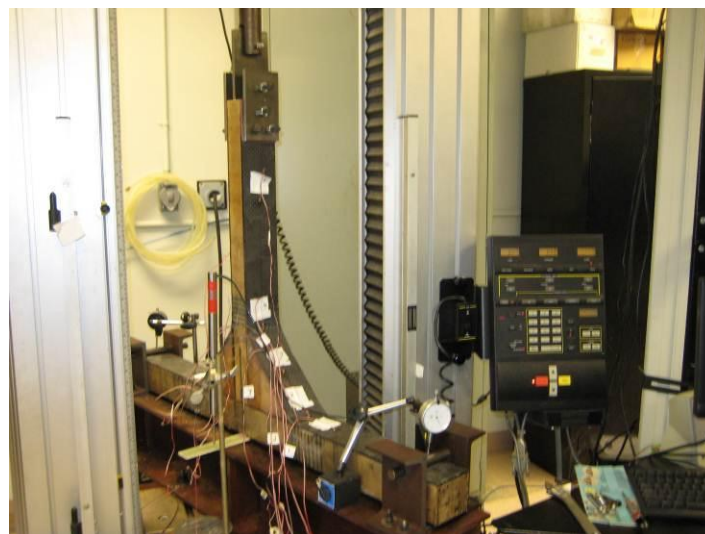
Fig. 16 Test set up for a T-Joint
