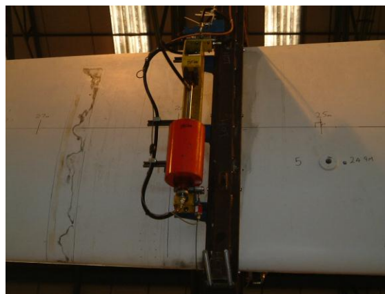
Fig. 13 Narec's ‘saddlebag’ resonant mass system
