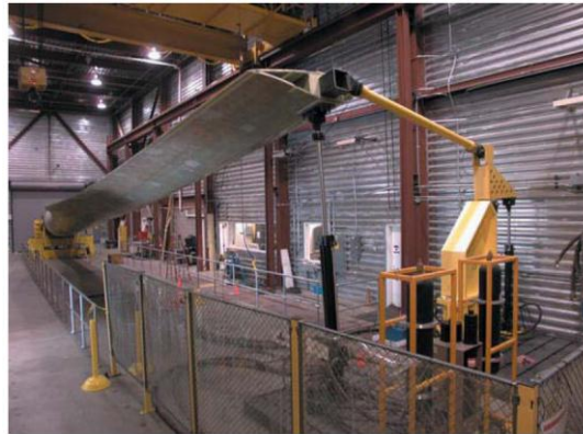
Fig. 16 Dual-axis test set-up using hydraulic actuator and side-mounted push-rod
