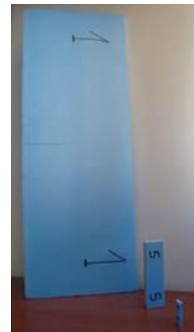
Fig. 35 Size effect samples
