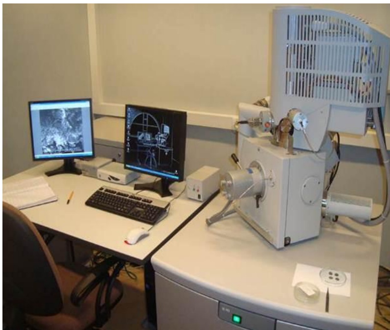
Fig. 45 Scanning Electron Microscope used for microstructural analysis
