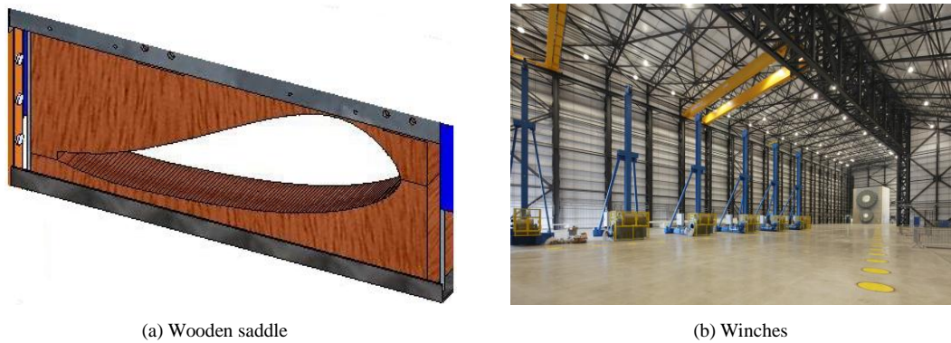
Fig. 8 Saddle and winches used in static testing of blade
