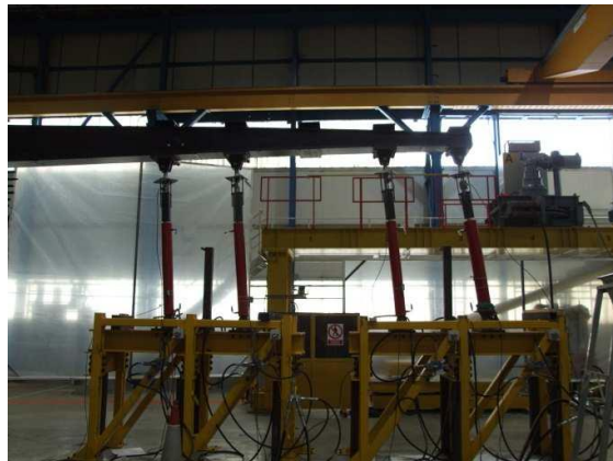
Fig. 6 Static testing of a marine turbine blade using hydraulic actuators
