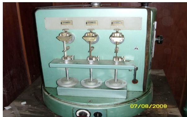
Fig. 1 Device for testing bending fatigue
