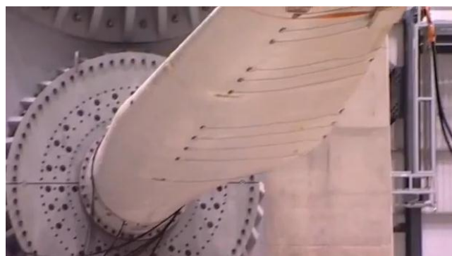
Fig. 29 The array of mechanical strain gauges in fatigue testing of a wind turbine blade
