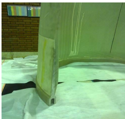
Fig. 4 Cross section view of root joint
