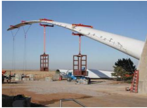
Fig. 5 Static testing of a long blade using ballast weights
