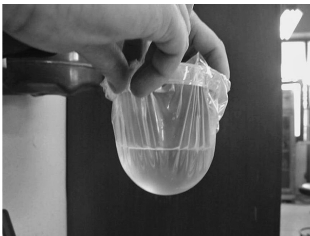
Figure 9.19 Starch/MMT/chitosan nanocomposite film with improved hydrophobic nature (Kampeerapappun et al., 2007).
