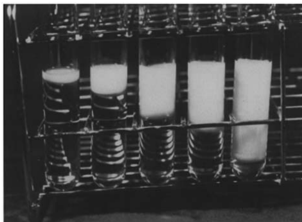
Figure 15. Bacterial cellulose layers grown with different culture time (max 4 weeks). 30 © Springer. Reproduced by permission of Springer. Permission to reuse must be obtained from the rightsholder.
