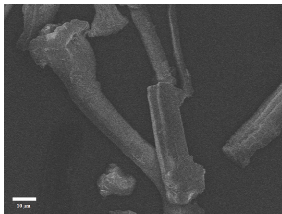
Fig. 5. SEM image of TSH (magnification: 1000 \times ).
