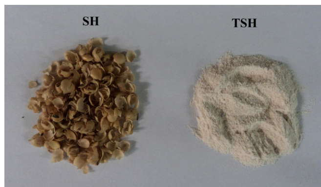
Fig. 1. Images of soy hulls before (left) and after the purification (right).
