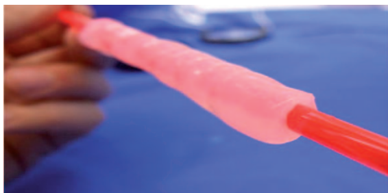
Figure 23. Tube of bacterial nanocellulose designed by a matrix technology and presented on a red glass rod, which symbolizes the blood flow when the tube is used as a blood-vessel substitute; inner diameter: 6 mm, length: 15 cm. [182]
