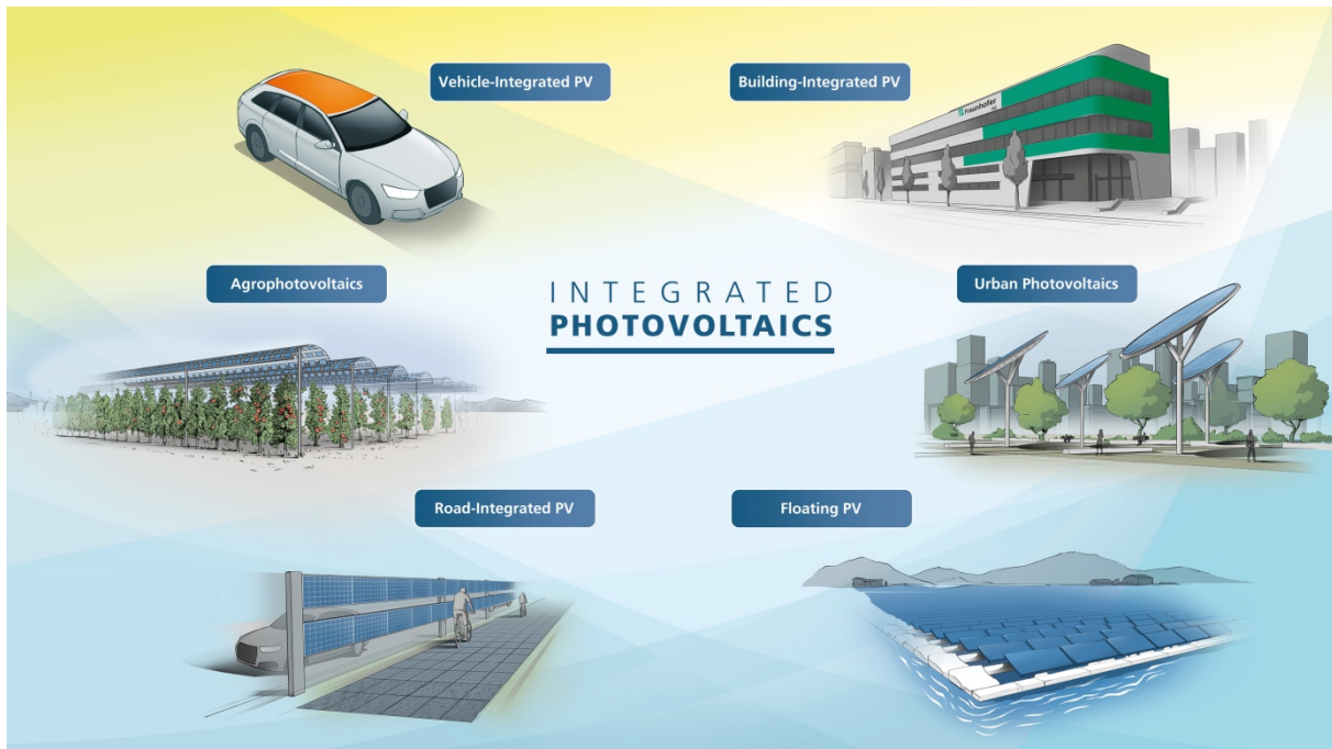
Figure 30: Applications for the integration of photovoltaic
