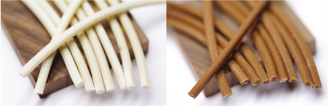
Above: Fraunhofer Institute researchers have produced a range of flame-retardant bio-filaments for 3D printing
