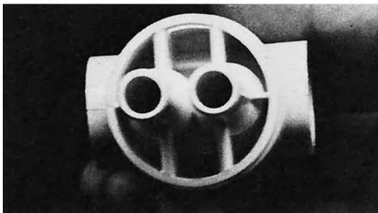
Figure 2 View of the exterior of the valve housing
