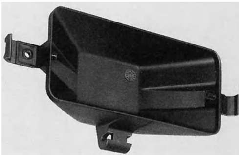
Figure 1 Lamp housing of polypropylene, reinforced with 15 wt.% glassfiber, flame-retardant
