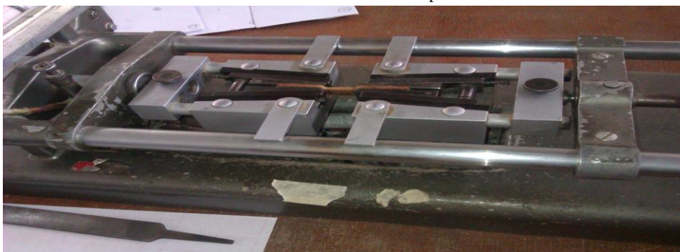
Plate 1. Tensile test experiment using tensometer equipment
