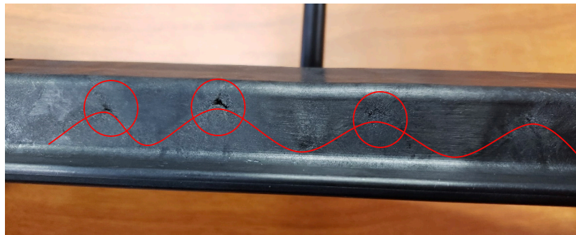
Figure 7: Air Gaps and Weld Lines
