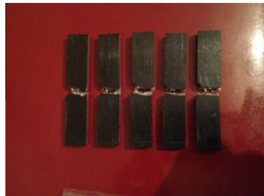
Fig. 26. Nano-strengthened hybrid composite impact specimens.
