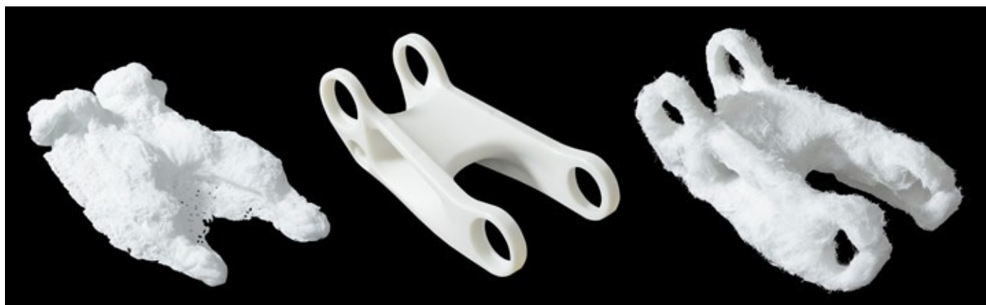
Left: Short-fiber internal fiber structure after resin removal. Middle: Injection molded part. Right: Long-fiber internal fiber structure.
