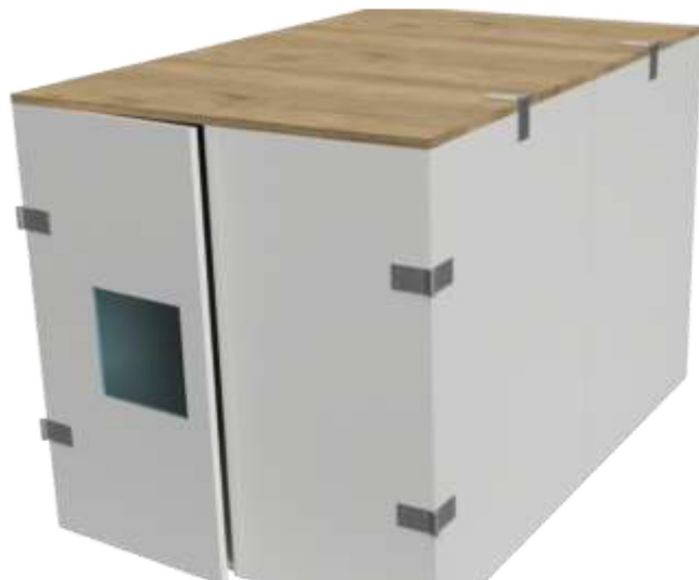
Fig. 10. Hinge placement for doors and top cover.
