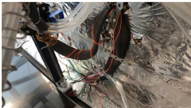
Fig. 71. Cable management for X axis and extruder.
