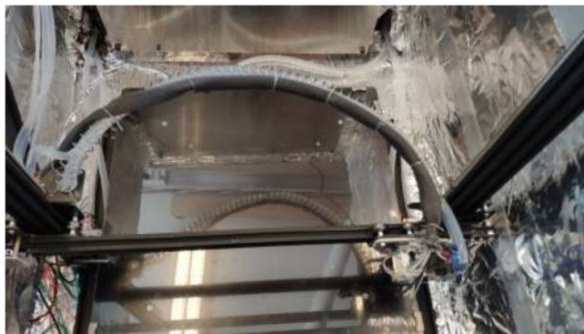
Fig. 70. Extruder cable management.
