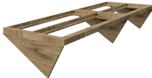
Fig. 26. Radiator holder support.
