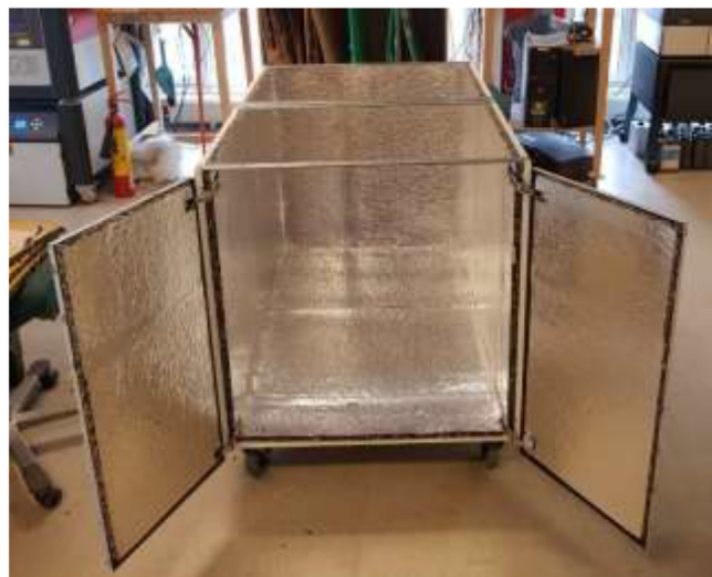
Fig. 11. Insulation of heated chamber.
