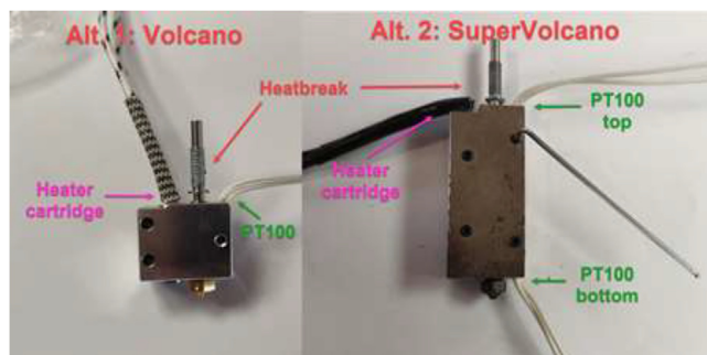
Fig. 43. Volcano (left) and SuperVolcano (right) hotend assembly.
