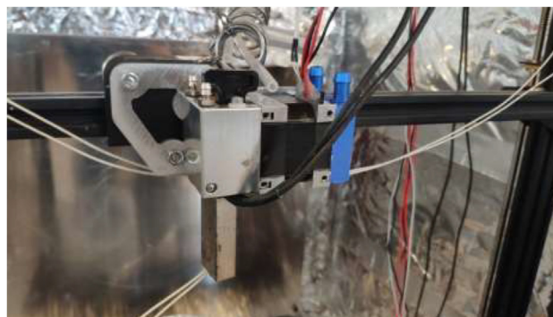
Fig. 56. Extruder installed on X-carriage.
