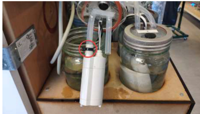
Fig. 98. Tube mounted using zip-tie to pump.
