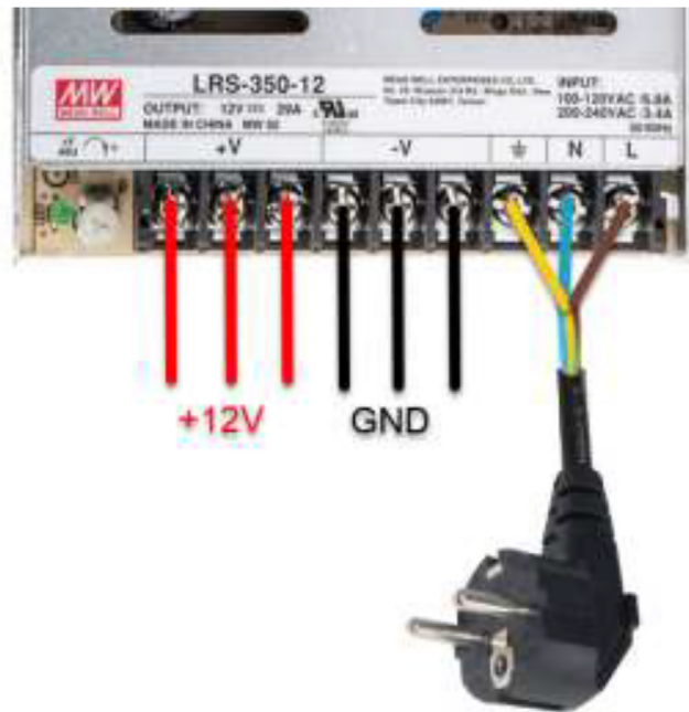
Fig. 78. 3D printer PSU wiring diagram [19,20]
