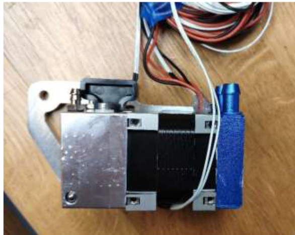
Fig. 42. TriangleLab Matrix Liquid-Cooled extruder.
