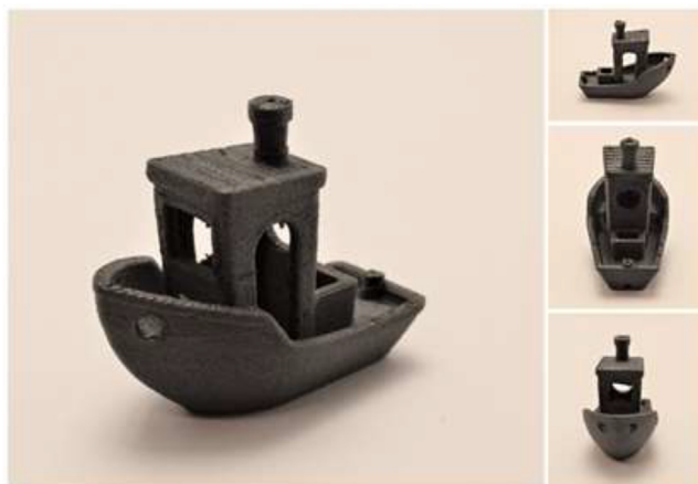
Fig. 138. 3DBenchy printed to showcase the geometrical details of printed CF-PEEK.
