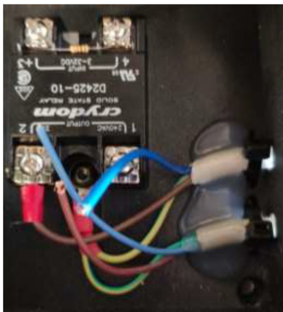
Fig. 124. Drying chamber strain relief.
