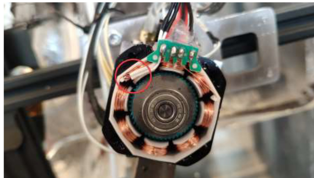
Fig. 39. Inserting thermistor for temperature observation.
