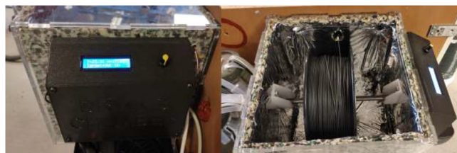
Fig. 125. Finished drying chamber.
