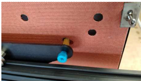
Fig. 46. Underside of heated bed with new bed leveling nut installed.
