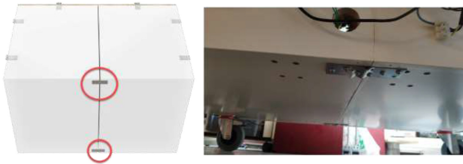
Fig. 5. Interconnection of two closets.
