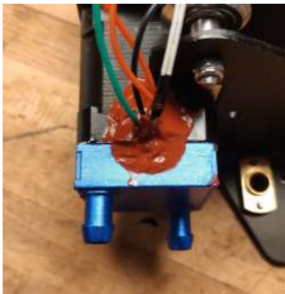
Fig. 41. Mount cooling block and add HTS.
