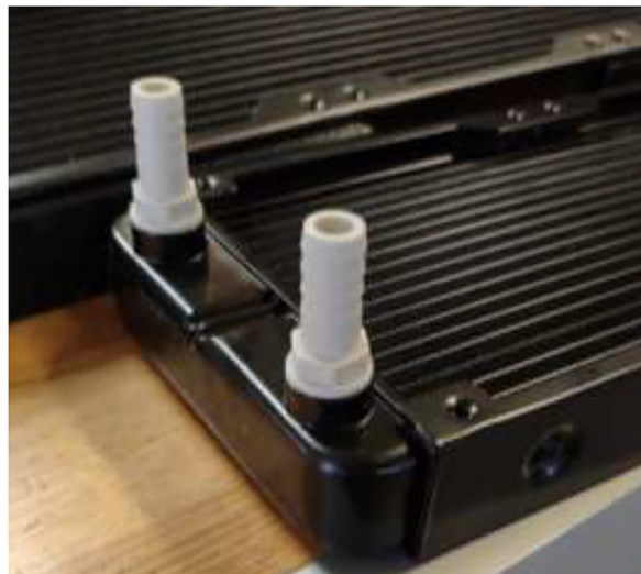
Fig. 108. G1/4" adapter installation.
