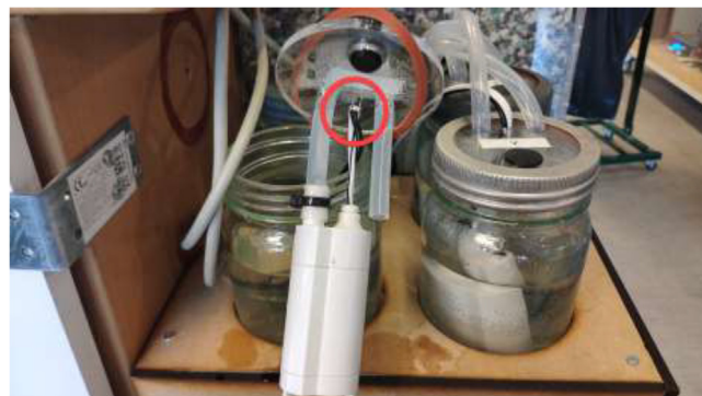
Fig. 88. Pulling cables through cover.
