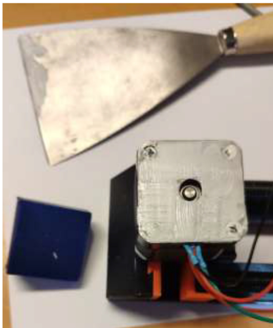
Fig. 40. Apply a thin layer of heatsink plaster after grinding and washing.
