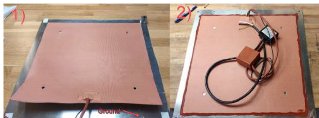
Fig. 17. Silicone heater applying steps. 1) Glue silicone heater and add grounding cable. 2) Add HTS around edges.
