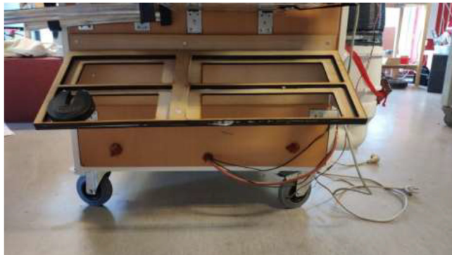
Fig. 28. Radiatorholder mounted on backplate.
