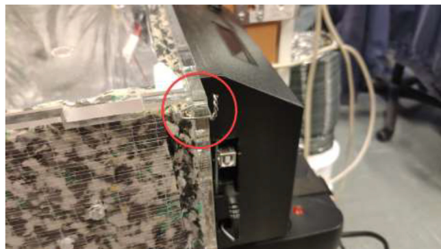
Fig. 114. Steel wire to assemble drying-chamber.
