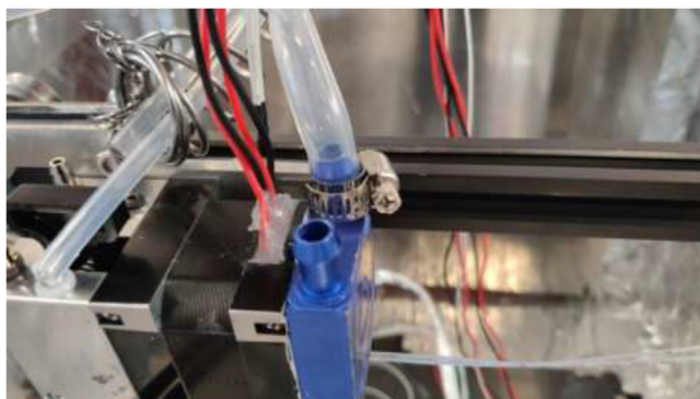
Fig. 102. Tube installed on extruder stepper-motor.
