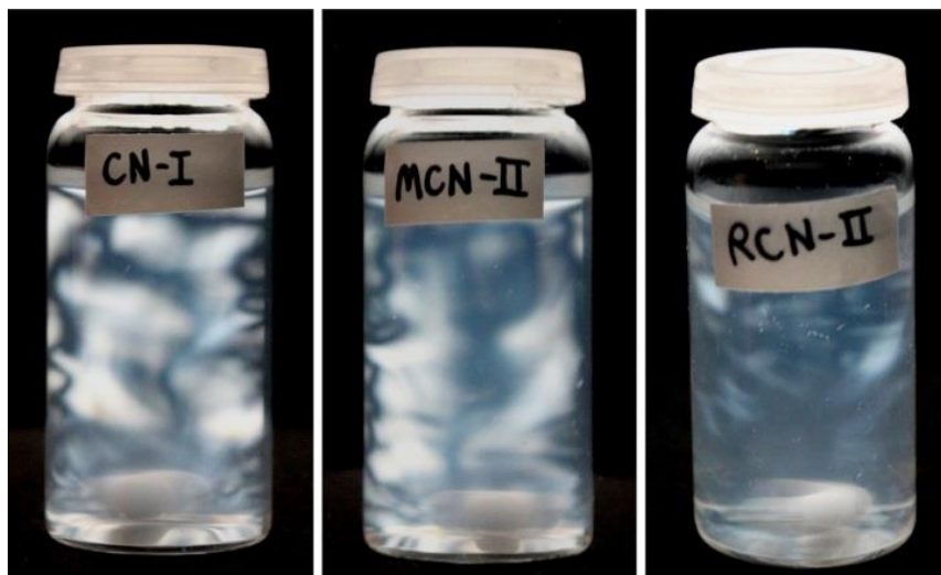
Figure S1 – Shear-induced birefringence for 0.15 wt% aqueous suspensions of cellulose nanocrystals under stirring, visualized between crossed polars.
