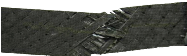
FIGURE 10: Shear tested specimen of multiscale composite.
