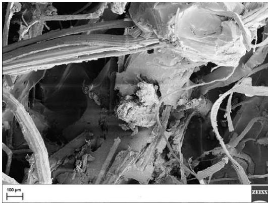
Fig. 8. SEM image of hemp/epoxy composite with 0% w/w lignin added.
