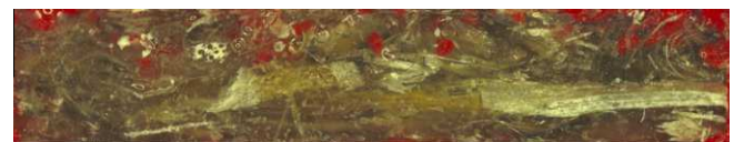
Fig. 12. Dark field optical micrograph of hemp/epoxy composite with 0% w/w lignin.
