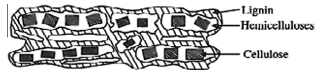
Fig. 3. Structural organisation of the three major constituents in the fibre cell wall [50].
