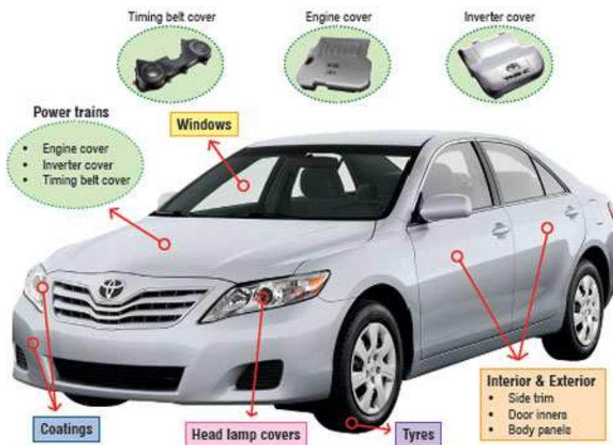
Figure 4.6: parts of car(Automotive), that nanocomposites are used in it
