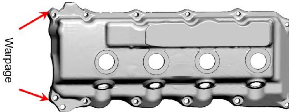
Figure 2: Simulation model of a cylinder head cover showing warpage locations
