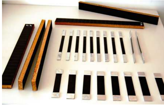
Fig. 1.8 Typical carbon/epoxy (CFRP) for tension loading and CFRP/honeycomb sandwich specimens for bending experiments
