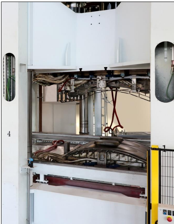
Production line set-up for sidewall moulding trials (Photo: Cannon Group)
