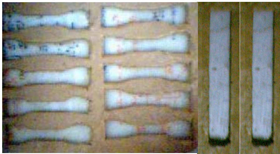
Figure 4-1 matrix sample produced from paste of panes rolled out at pane and then formed the shape of tensile and bending tests.
