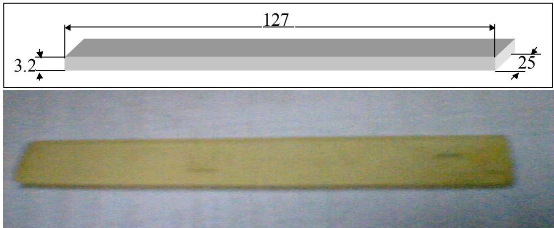
Figure 4-4 Matrix Flexural test specimens
