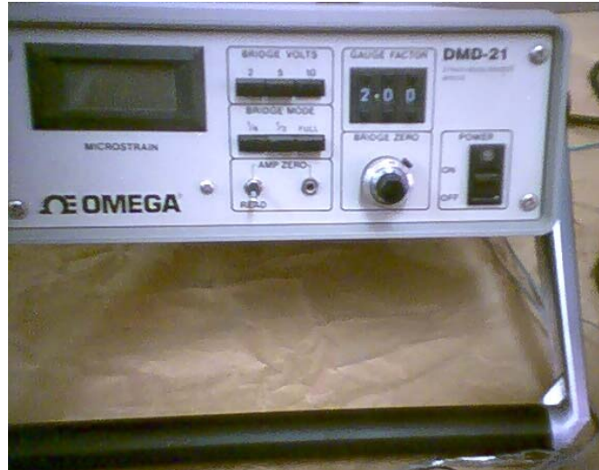
Figure 4-9 Micro Strain meter used in tensile tests.
