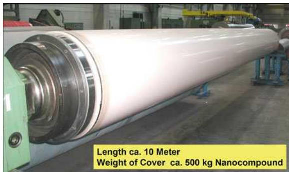
Fig. 6.34 A large calender roller, freshly covered with a newly designed nano-compound
