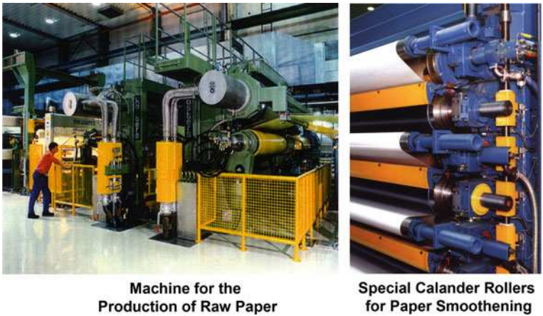
Fig. 6.33 Numerous calender rollers in a huge paper making machine
