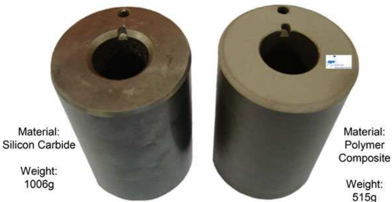
Fig. 6.32 Comparison of the new composite bearing ( right ) with the existing one made of monolithic SiC ( left )
